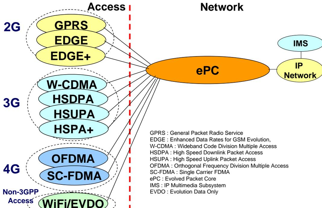
Figure 4 : ePC : Convergent packet core network
