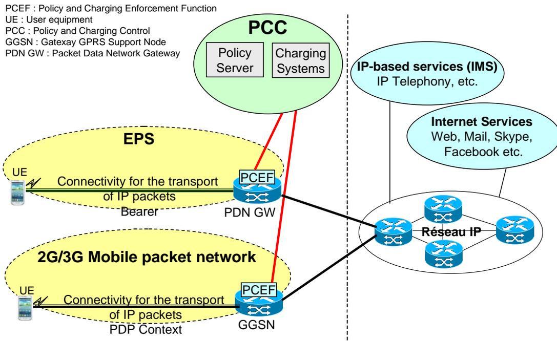
Figure 6 : PCC architecture for mobile data
