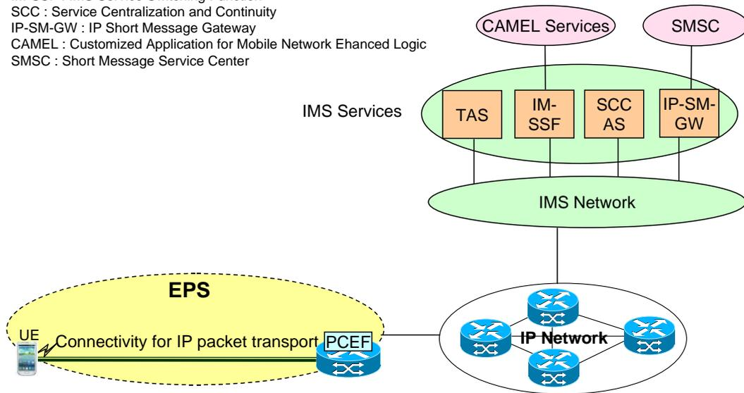
Figure 8 : VoLTE solution with IMS architecture
