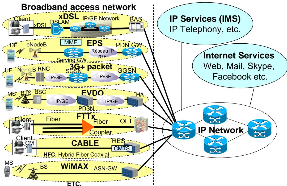
Figure 5 : IP-based Service Architecture and Broadband Access
