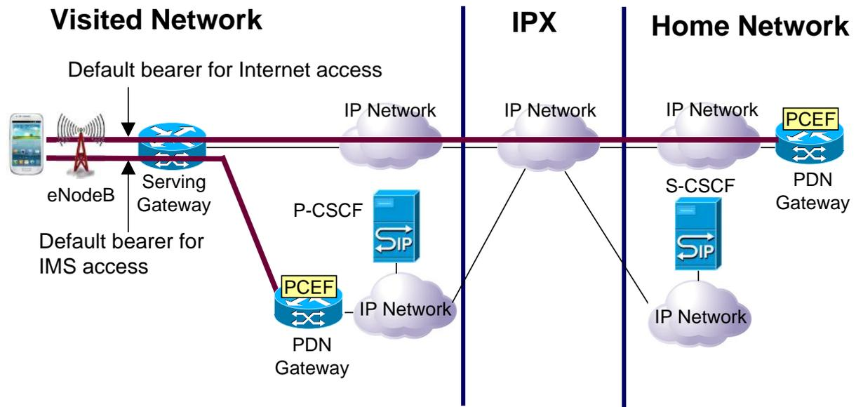
Figure 6 : Connectivity for Internet Access and IMS access when the user is in a roaming situation
